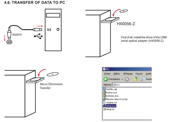
Then install the "Micro Ohmmeter Transfer" application software as explained in readme.txt.
