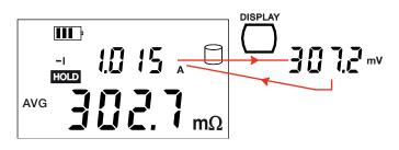
To display the voltage on the terminals of the resistance instead of the measurement current, press the DISPLAY key.
