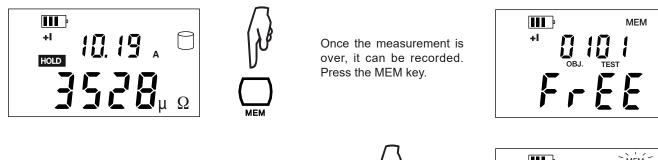
The instrument proposes the first free location in memory. If it is acceptable, execute a long press on the MEM key. To change the number of the test or of the object, use
