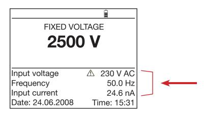
The insulation measurements cannot be started if there is an excessively high external voltage on the terminals, in which case the  $\triangle$  symbol is displayed next to the measured external voltage (see § 3.2).
