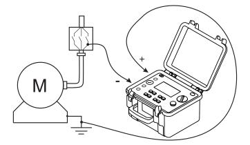
**To measure high insulation values (> 1 GΩ)**, we recommend using guard terminal "G" to avoid leakage and capacitive effects or eliminate the influence of surface leakage currents. The guard terminal is connected to a surface where leakage currents may flow through dust and humidity, e.g. the insulation surface of a cable or transformer, between two measurement points.
