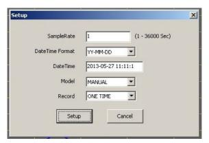
To set the data sampling rate, date and time format as shown above, click the 'Data Logger' tab and choose 'Setup'. Other settings can be left as default.
