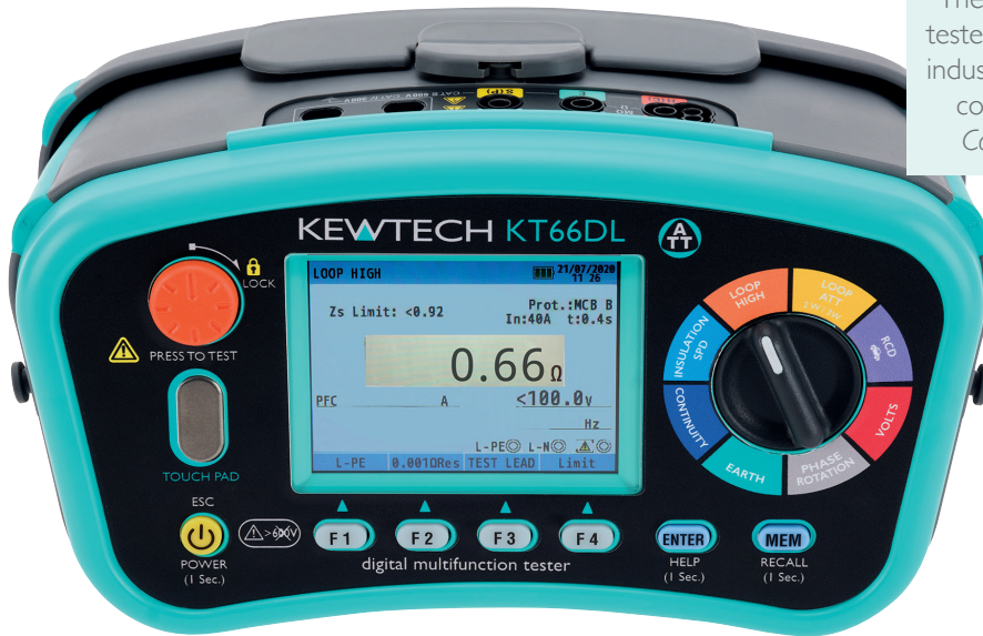
Large full colour screen, here showing a high current 2 wire 3 digit resolution loop impedance test with max Zs reference also displayed.
