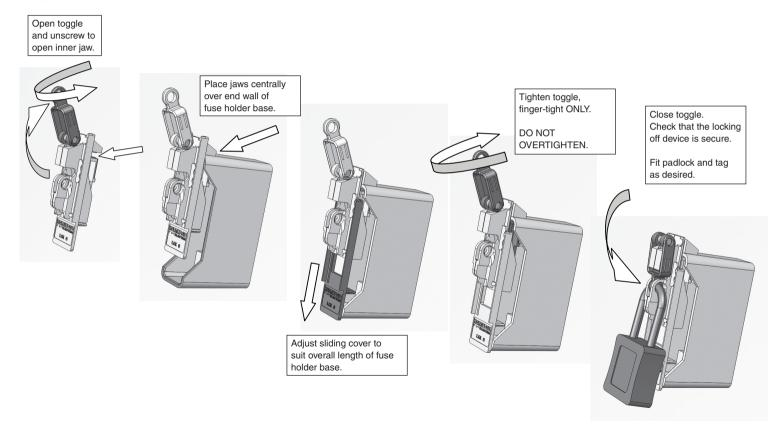
All models are quick to install without the need for any tools. The construction is all insulating plastic, without any metal parts, to reduce the risk of use in live working environments.
