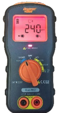
Fault condition missing earth
