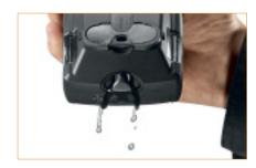
The measurement values can be read off on the well-lit display. The testo 310 has a battery life of 10 hours. It is excellently suited to rough surroundings. The condensation trap can be emptied quickly and easily.
