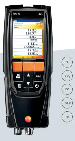
Designed especially for the UK market, the testo 320B has a colour graphic display providing a unique user interface experience to access measurement menus for:
