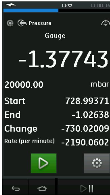
Figure 2-27 Leak Test Example
